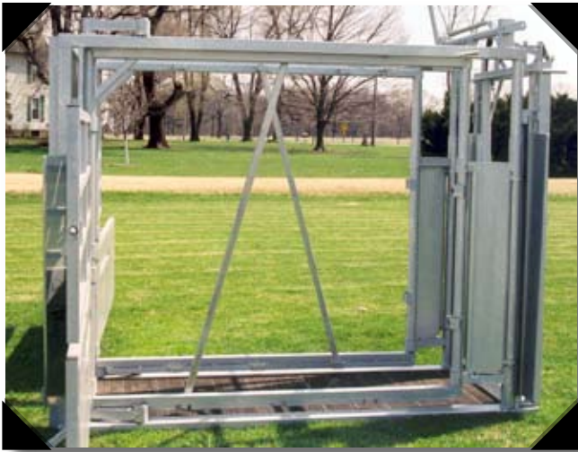
Variable position vertical bars move with the squeeze side frames
